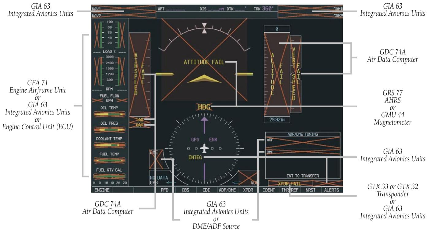
Figure 4 G1000 System Failure Indications
